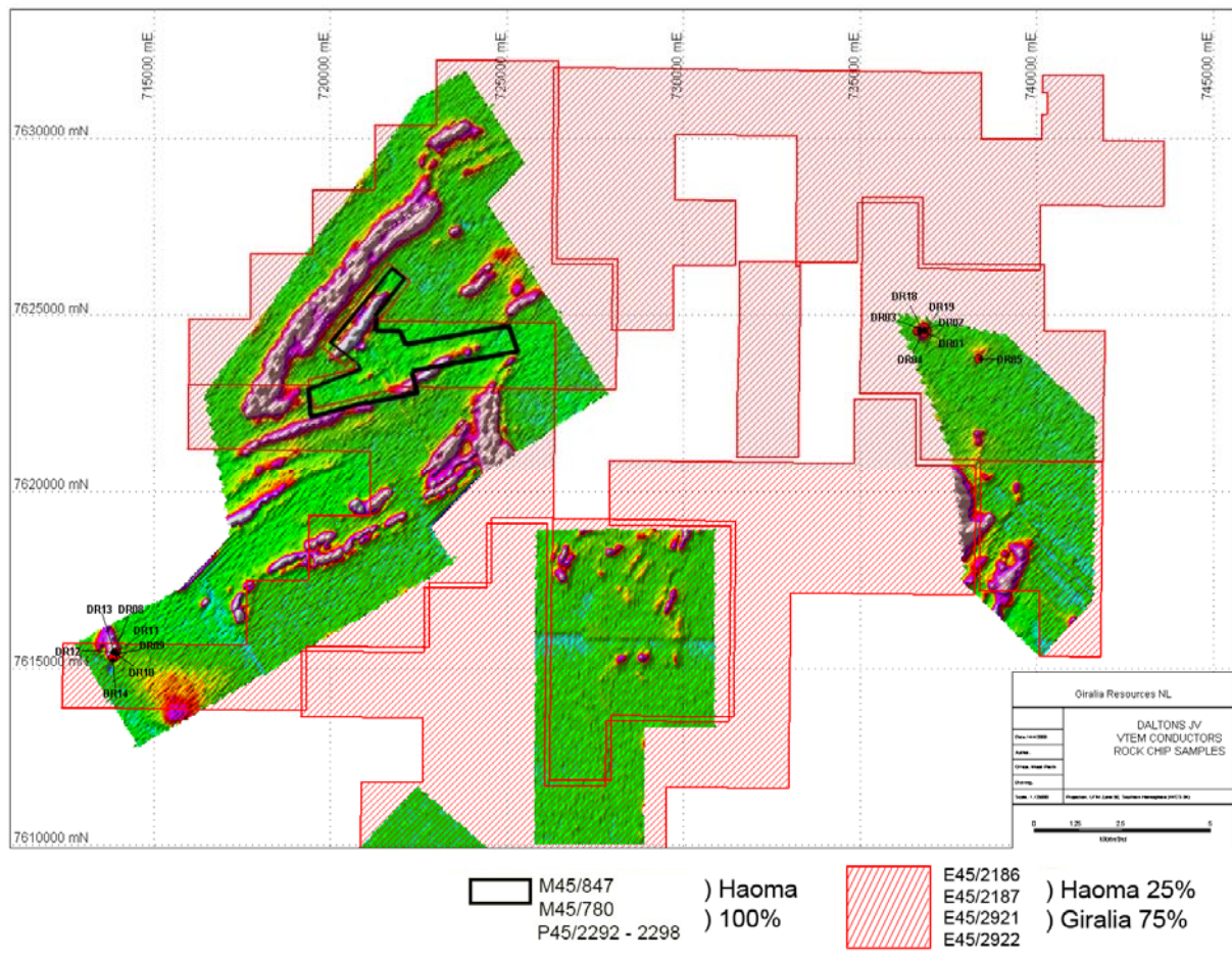
Figure 2: Daltons area; Late time VTEM conductors (Giralia JV tenements in red) Showing March 2008 rock chip sample locations
