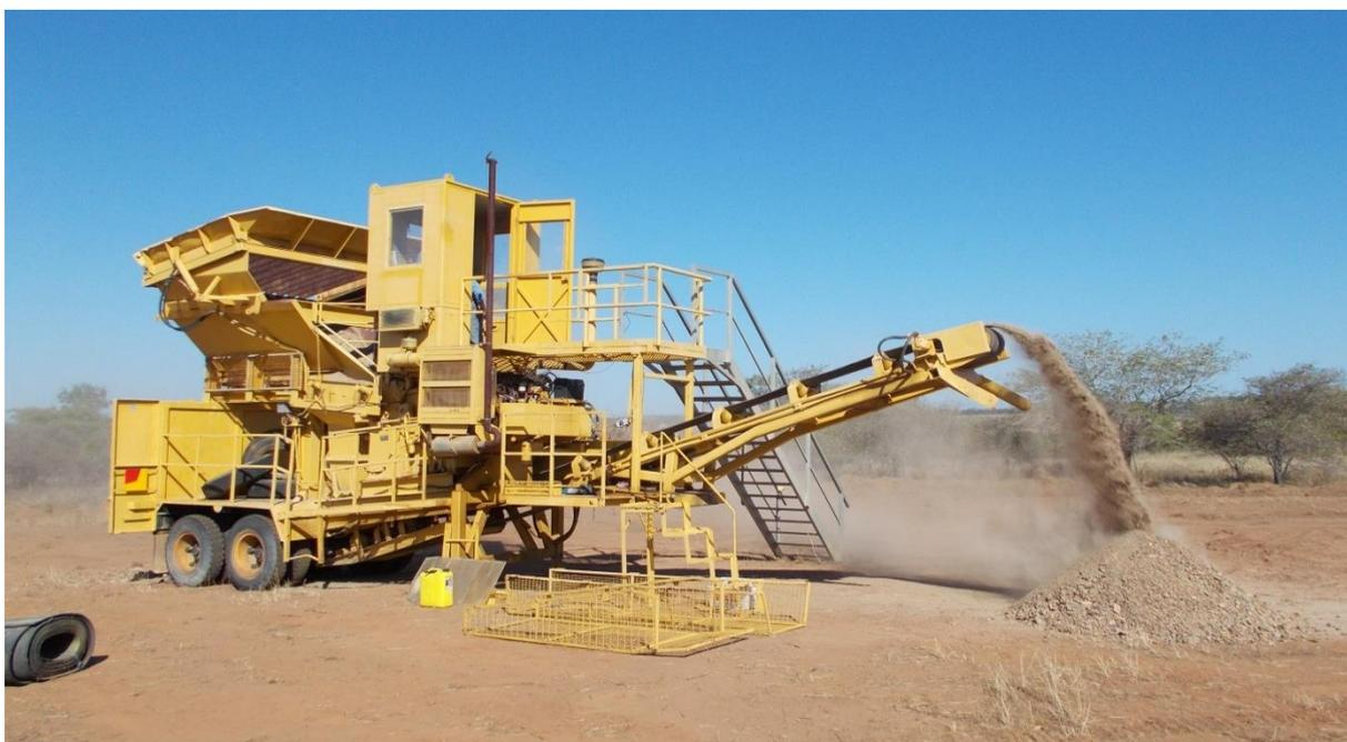
**Figure 4: Haoma's Ravenswood Mobile Crusher being tested during commissioning at Copper Knob (ML1330)**
